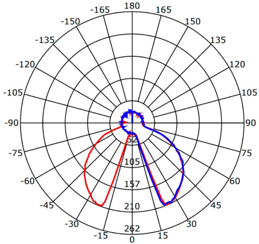
Beam Angle(50%) C0-180,C90-270: 120.6 deg,44.5 deg
